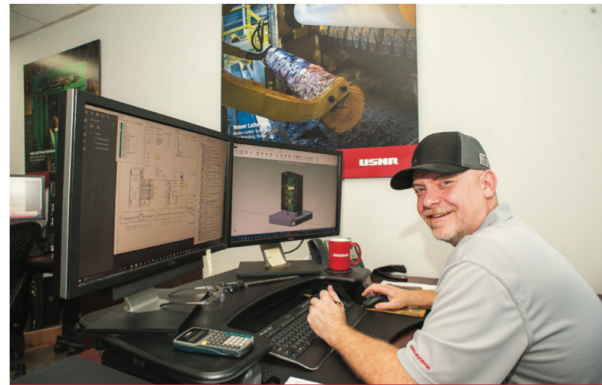
CNC programmer Adam Corson proves parts in Mastercam so that operators can confidently run machines lights out.
